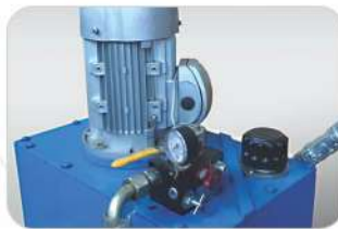
Power Pack Unit
